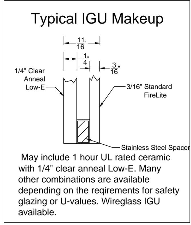
See Fire-Rated Glazing Section for various options and configurations for U.L. labeled glazing.
